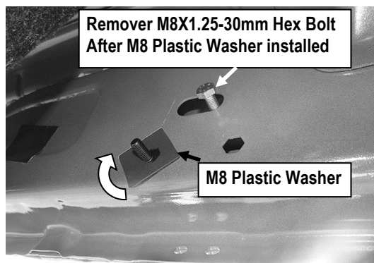
(Fig 5) Thread Plastic Retainer Onto the Welded Bolt on M8 Bolt/Nut Plate To Hold Bolt/Nut Plate In Position.
