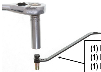
(Fig 8) M8 Rivet Insert Installation Tool Assembly
