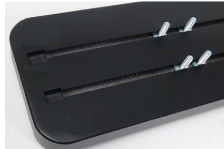
(Fig 8) Slip (2) M6X1-20mm Square Head Bolts Into Each Bottom Channel
