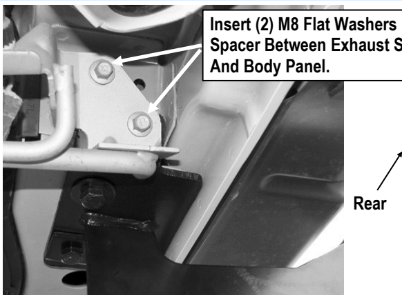
(Fig 11) Passenger Rear Mounting Bracket (09-010 models: Install Mounting Bracket Between Exhaust Support And Body Panel )
