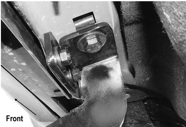
(Fig 4) Passenger Front Mounting Bracket Installation
