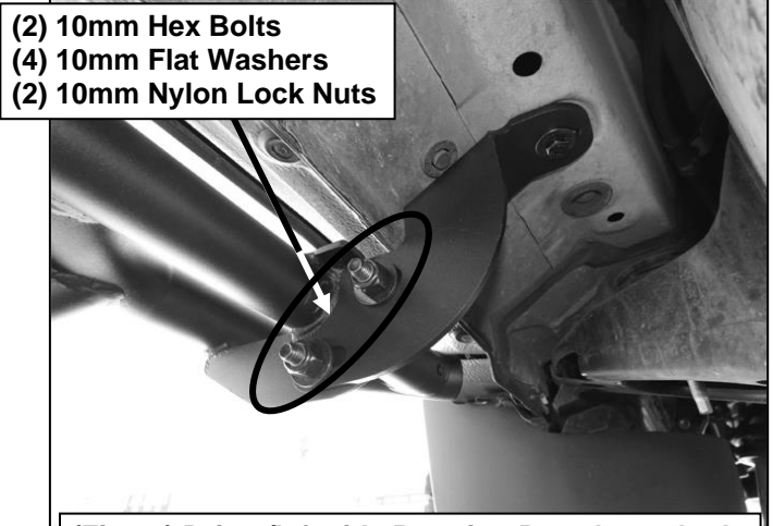
(Fig 13) Driver/left side Running Board attached to the front facing side of the front Bracket
